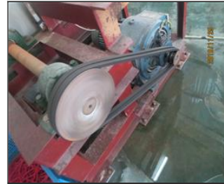
Photo of non-conformity NC 7.17 The cutting machine in the workshop were not equipped with pulley guard.JPG
