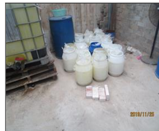
Photo of non-conformity NC 7.6 No label or anti leakage facility for chemical.JPG
